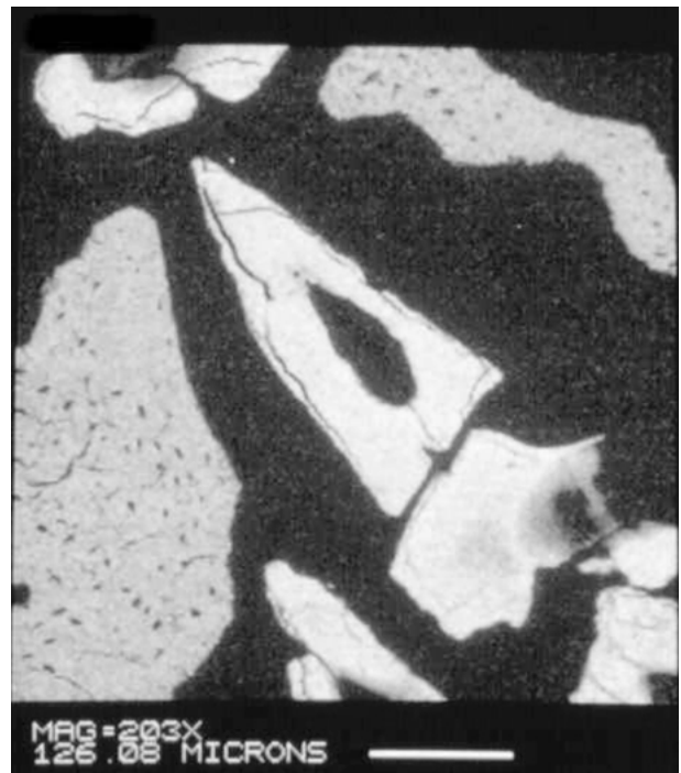
Figure 10 The SEM-image of a bioactive glass particle after six months of implantation.
